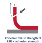
2. Test of adhesion strength by peeling test
