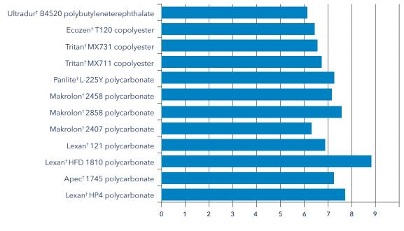
Peeling Force Avg. (N/mm) 24 h at RT Note: Test data. Actual results may vary. Test specimen molded with injection molding and subjected to an additional storage for 24 h at RT. Molding conditions: 100 sec at 130 °C. <sup>1</sup> In accordance to DIN 53268.
