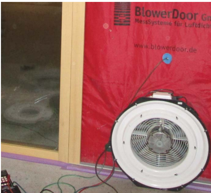
On-site air-leakage testing
